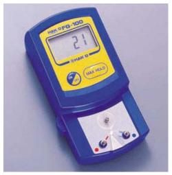
verification or calibration processes. When the MAX HOLD feature is enabled the thermometer will display the maximum temperature measured. To preserve battery life the auto shutoff feature turns the thermometer off when not used for three minutes. The thermometer design allows for easy measurements from right or left handed operators.
