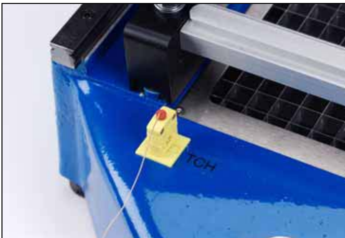
Figure 6: Thermocouple Inputs (TCH Shown)
