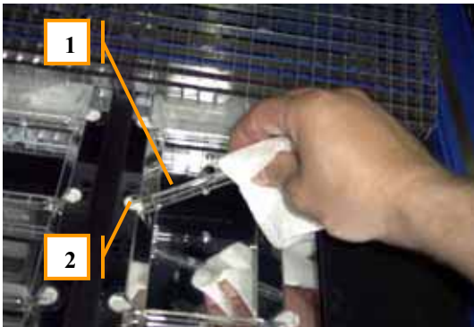
Figure 33: Replacing the bottom heater quartz lamps
