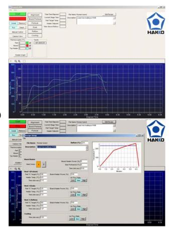
controllable for the Cool stage. Recipes can also be set that include a bottom side preheat to a selected temperature prior to the Preheat stage. Teach mode profiling sets the recipe times based on the input operating and target temperatures. PCs with a video capture card can view the CCD image from the FR-1418 on the computer.
