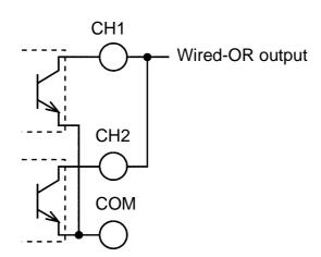
**Using on Wired-OR Logic**
