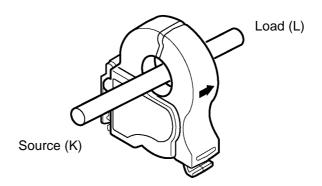
❖ See the "Connection diagram"(P.151) and refer to the instruction manual for the clamp sensor being used.
