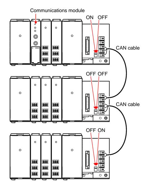
Connect Hi to Hi and Lo to Lo of the module bases. Only the CAN termination switch located on either side (a total of two) should be turned on. After all connections have been completed, check to make sure that the resistance between Hi and Lo is approx.  $60~\Omega$ .
