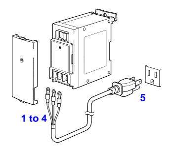
Connect the cable leads as shown below (at tightening torque of 0.8 N•m).
