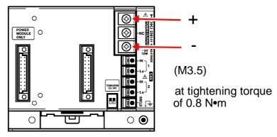
For the power supply output cable, use a cable with a conductor cross section of 0.75 mm<sup>2</sup> (AWG18) or more and length of up to 1 meter.
