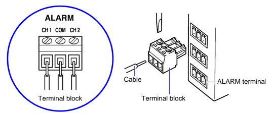
Connect the cable for CH1 output to CH1 and COM; connect the cable for CH2 output to CH2 and COM.
