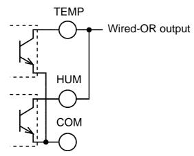
**Using on Wired-OR Logic**
