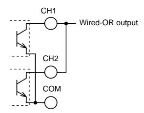
**Using on Wired-OR Logic**
