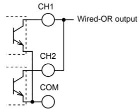
**Using on Wired-OR Logic**
