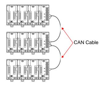
Connect Hi to Hi and Lo to Lo of the module bases. Only the CAN termination switch located on either side (a total of two) should be turned on. After all connections have been completed, check to make sure that the resistance between Hi and Lo is approx. 60  $\Omega$ .
