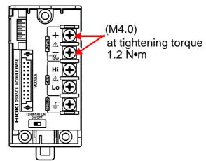
For the power supply output cable, use a cable with a conductor cross section of 1.0 mm<sup>2</sup> or more and length of up to 1 meter (3.28 feet).
