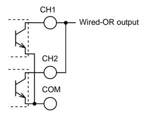
**Using on Wired-OR Logic**
