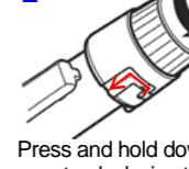
Press and hold down the switch, then turn it counterclockwise to remove the switch section.
