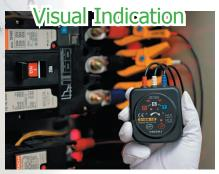
Based on the electrostatic induction theory, the 3129 series Phase Detectors can safely and accurately detect phase rotation in three-phase circuits. Correct rotation is indicated by a crystal clear beeping tune, while bright red LEDs show rotation direction.
