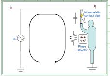
Non-contact phase detectors offers safe and correct phase detection based on the basic understanding that a closed circuit is formed between the conductor, detecting device and the operator with reference to the earth.
