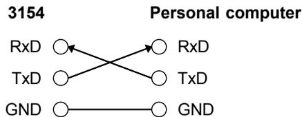
Cable connector on the unit Wiring: Reverse wiring
