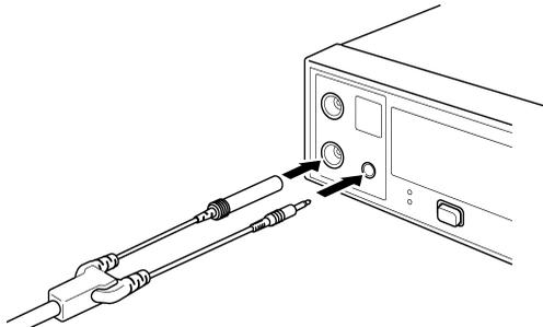
When disconnecting 9299 from the 3154, disconnect test probe first and signal lead last.
