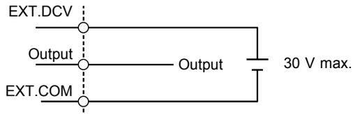
(3) When using internal DC power, the signals between INT.DCV and EXT.DCV, and between INT.GND and EXT.COM will both short circuit, and HIGH (5 VDC) and LOW signals are available between the output and INT.GND terminals.
