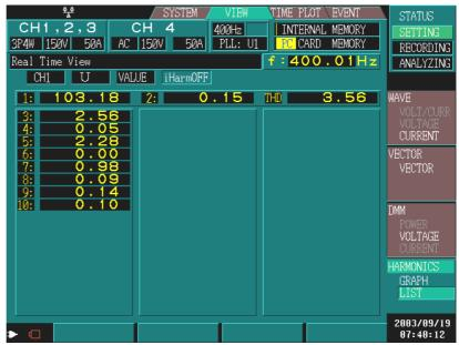
In the harmonics bar graph and list screens, the harmonics from the fundamental wave (1st) to 10th orders are displayed in 400Hz mode.
