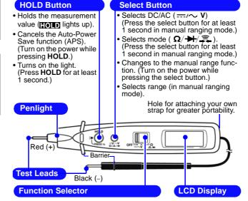
OFF Power Off (Power is turned ON in any position other than OFF.)
