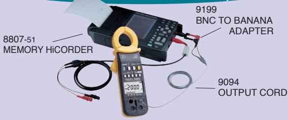
Using the external output functions of the 3284 or 3285 in combination with a HIOKI MEMORY HiCORDER enables recording of current and frequency fluctuations and recording and harmonic analysis of instantaneous waveforms. The monitor output (MON) spans a wide frequency range from DC to 20 kHz (15 kHz in the case of 3285), which allows the units to be used for electric current analysis in various fields ranging from batteries to inverters.
