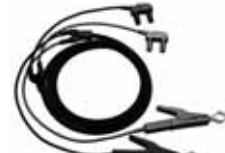
9467 LARGE CLIP TYPE LEADS (Cable length: connector to fork 85 cm, fork to probes 25 cm; maximum clip diameter 29 mm)
