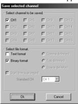
(2) Select channels to be saved and saving file format. Select [**OK**] to proceed with selecting file names and destination for saving.
