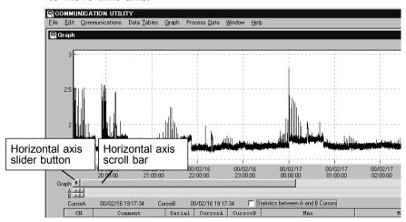
Click vertical axis slider button or drag vertical axis scroll bar to move vertical axis.
