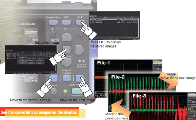
Save important waveform images instantly with the press the press of a button. Review images by flipping through each file on the widescreen display.
