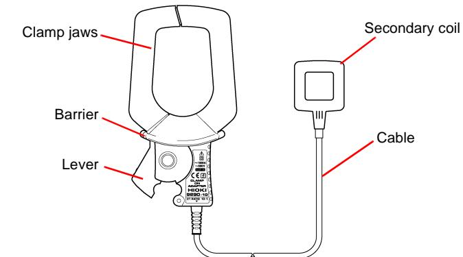
The clamp sensor and secondary coil are marked to indicate the direction of current flow, to ensure that the measurement current and output current have the same phase.
