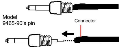
5. Replace the 9465-90 pin tip by inserting a new pin into the socket and pressing against a hard board or other surface to fix the pin firmly in place.
