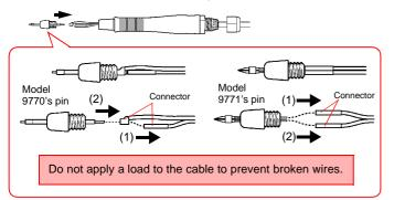
**5.** Fasten a new pin. Press the tip of the pin against a desk so that the pin won't spring out, and push the connector onto the pin.
