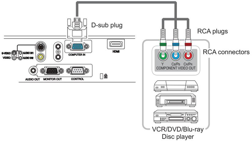
To input component video signal to the **COMPUTER IN** port of the projector, use a RCA to D-sub cable or adapter.
