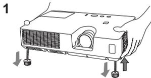
To loose an elevator foot, pull up the elevator knob on the same side as it.
