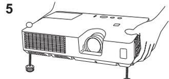
To finely adjust, twist the foot.
