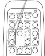
1. Press the **MAGNIFY ON** button on the remote control. The picture will be magnified, and the MAGNIFY dialog will appear on the screen. When the **MAGNIFY ON** button is pressed for the first time after the projector is turned on, the picture will be zoomed by 1.5 times. On the dialog, triangle marks to show each direction will be displayed.
