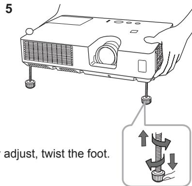
To finely adjust, twist the foot.
