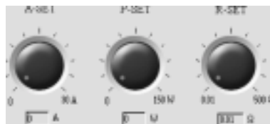
Fig.2-4 (1) Setup the Current Value, the Power Value and the Resistance Value Using Rotary
