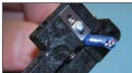
Score cable with stripper CAT. NO. 45-165
