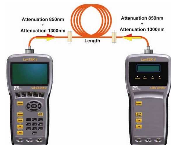
Figure 5: FiberTEK® FDX bi-directional testing without mandrels
