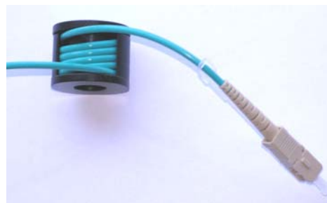
Figure 3: Fiber optic mandrel wrap
