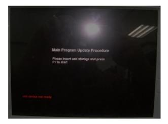
4. When the **xxx.opg** file on USB flash disk has been recognized by oscilloscope, the message "**usb device ready**" will appear on the lower left corner.
