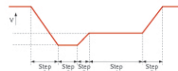
Voltage fluctuation test pattern
