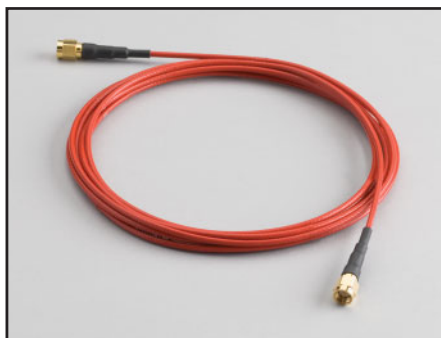
CA-446A: 3m (9.8 ft) coax cable terminated with an SMA male plug on each end, 100Ω impedance.
