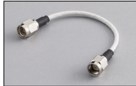
CA-451A: 10.8cm (4.25 in) RG188 coax cable terminated with an SMA male plug on each end, 50Ω impedance.
