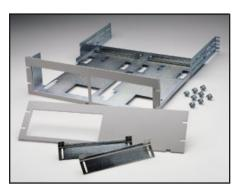
Model 4288-5 Fixed Rack Mount Kit: The single- and dual-instrument front panels included enable rack mounting of either one or two 3½-inch instruments. Height: 132mm (5¼ in). Depth: 457mm(18 in).
