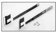
Model 1939 Slide Rack Mount Kit: Consists of two sets of flanged brackets, equipment slides, and hardware for mounting the Model 237 in a standard 48.3cm (19 in) equipment cabinet. Can be used with Model 8000. 89mm (31/4 in) height.
