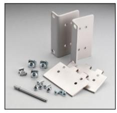
Model 4299-4 Universal Dual Unit Rack Mount Kit: Includes all required hardware to rack mount two Keithley and/or Agilent half-rack instruments together using front panel only mounting into a standard 19-inch equipment rack. Not compatible with Series 2600A. 88mm (3.5 in) height.
