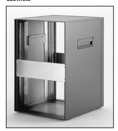
Model 8000: A 28-inch high equipment cabinet that is open on both ends. It accepts all Keithley rack mounting kits as well as most rack kits provided with other instrumentation. The dark brown 8000 comes fully assembled, with handles permanently installed on each side. One hundred chrome Phillips head screws with mylar washers and clip nuts are provided for instrument mounting. Rack mounting kits are available separately.
