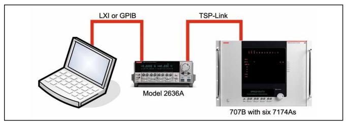
Series 2600A SMUs have an on-board test script processor (TSP) that executes test scripts and controls the switch matrix via the TSP-Link, which acts like a hardware backplane, connecting the two high-performance processors at full hardware speeds. This configuration provides the best possible throughput and flexibility and the tightest synchronization between the instrument and the switch matrix.
