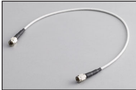
CA-406B: 33cm (13 in) RG188 coax cable terminated with an SMA male plug on each end, 50Ω impedance.
