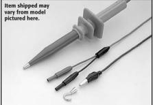
Model 1600A High Voltage Probe MAXIMUM INPUT: 40kV DC or peak AC to 300Hz. INPUT RESISTANCE:  $1000M\Omega$ . DIVISION RATIO: 1000:1 (into  $10M\Omega$ ).
