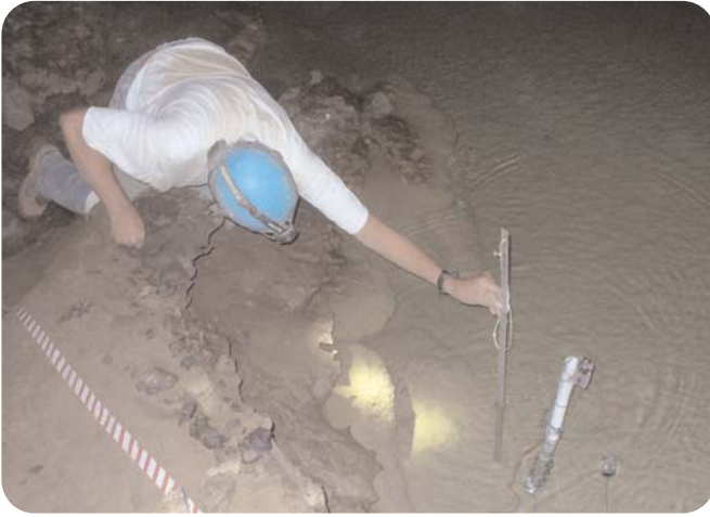
Steve Peerman measuring water depth next to sensor. John McLean photo.
