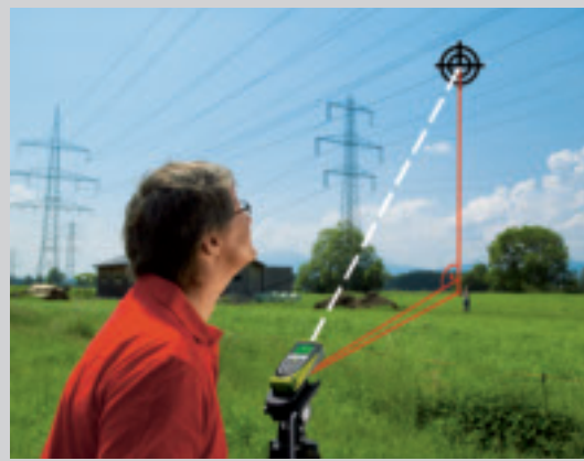
Indirect height measurements by using the tilt sensor and the digital viewfinder, heights can be determined with the first measurement even without reflecting the laser beam.
