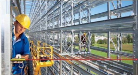
Storable – measuring long range distances with the digital Pointfinder
