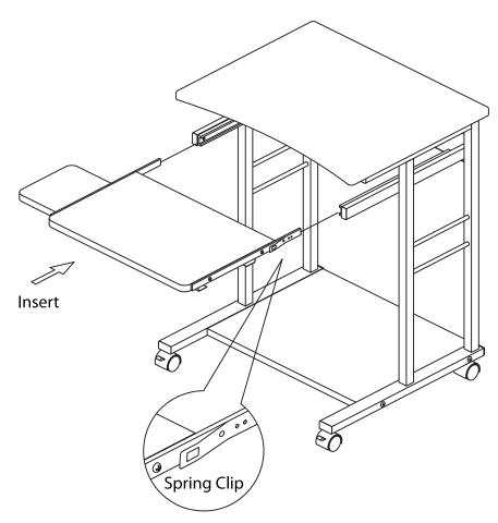
Push the spring clip to release the pull out shelf from the main unit.
