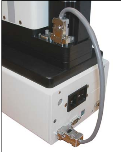
The illustration above depicts proper connection of the controller cable
