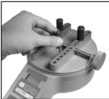
Fig. 1 Posts can easily be moved between holes
