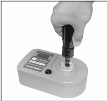
Fig. 1 Gradually exert torque to achieve accurate results
