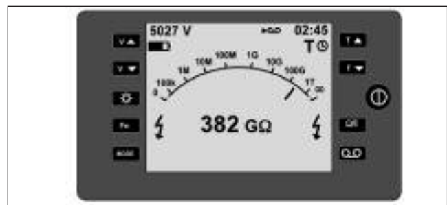
Figure 8: Megger MT520 Display
