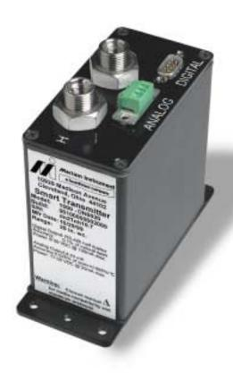
Meriam's 1500 Digital Transmitters are for high accuracy applications for OEM's, on manufactured skids, in process control systems and plant instrumentation. RS-485 communications allows for easy configuration using a PC or laptop computer. The RS-485 addressable interface allows up to 32 devices to be networked together. Optional 1-5 Volt or 4 - 20 mA outputs are also configured from a PC or laptop.
