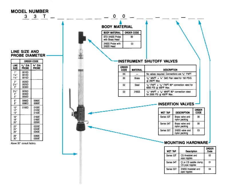
SERIES 33T ACCUTUBE PROBE AND WET TAP MOUNTING ASSEMBLIES. Use of the 33T allows insertion and removal without process shutdown. The 33T probe consists of standard brass head and 316SS probe and installs through a wet tap assembly. The wet tap assembly consists of a packing gland, pipe nipple,
