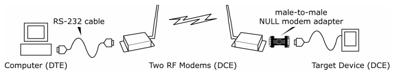
Figure 2.5. Typical wireless connection used for serial communications between DTE and DCE devices
