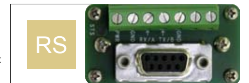
RS-232 / RS-485 communication connectors
