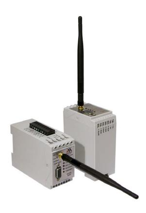
Meriam Industrial Wireless utilizes Frequency Hopping Spread Spectrum (FHSS) technology to hop to the different frequencies within the 902 to 928 MHz band.
