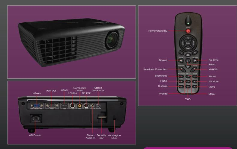
Small, sleek and stylish, the Optoma PRO350W provides a combination of performance and affordability. Features such as widescreen display, 2800 ANSI lumens, contrast ratio of 3000:1, lamp life of up to 4000 hours, filter-free design and low standby power consumption ensure that the Optoma PRO350W will not only save money in the long run, but also present a perfect, colorful, crisp image whether projecting a presentation or movie.
