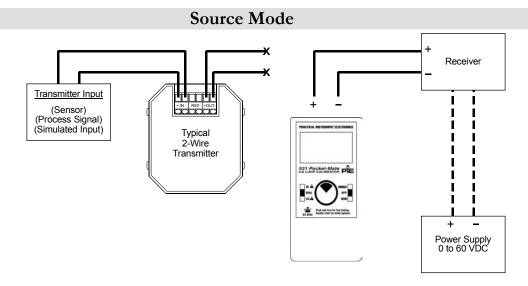
Source mode uses internal power to supply current from 0.00-24.00 mA into as much as  $1200\Omega$  until the end of battery life. The calibrator Graph will flash if connected improperly. The three-position EZ-Check switch provides instant preset 4mA at zero, 12mA at mid range and 20mA at full scale outputs. The output is adjusted in 0.01 or 0.10 mA increments (0.1 or 1.0) % display units with the EZ-Dial knob.
