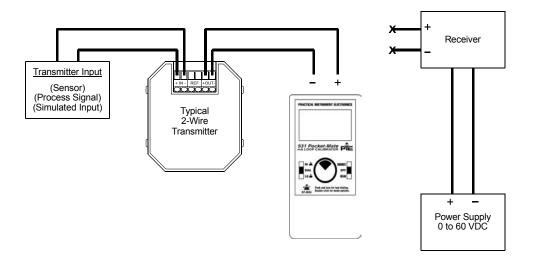
The Model 531 supplies 15Volts or 24 Volts to the transmitter and displays the output in mA or % on the Model 531 display. In read mode press the EZ-Dial™ Knob twice to get into the feature options. Then press the EZ-Dial™ Knob to select mA PWR - M. Then turn EZ-Dial™ Knob to select power range (15V or 24V). The EZ-Check switch and EZ-Dial knob allow rapid and fine control of loop current.
