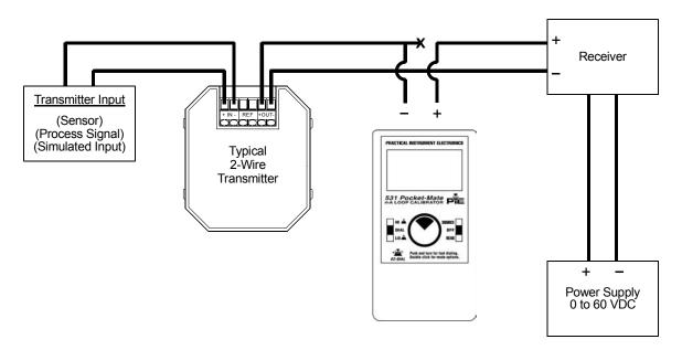
The Model 531 can read loop currents from 0-24 mA. The Model 531 limits current in read mode to 25mA to protect the devices in the loop from over voltage or over current conditions.
