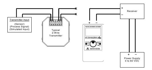
The Model 531 can simulate a 2-wire transmitter in the 4-20 mA or % process loop. In source mode press the EZ-Dial™ Knob twice to get into the feature options. Then press the EZ-Dial™ Knob to select mA 2 - wire. The EZ-Check switch and EZ-Dial knob allow rapid and fine control of loop current.
