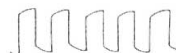
(c) Capacitance excessive
