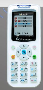
The teacher remote can directly communicate with student remotes without a computer via radio frequency.
