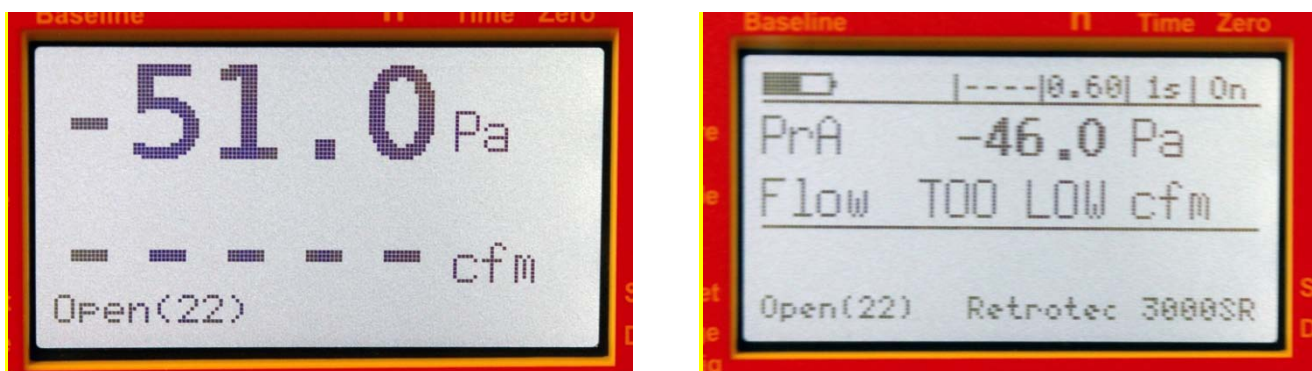
Figure 11. DM-2 can't display flow reading because of back pressure.
