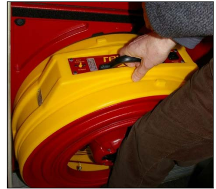
Figure 19. Installing a fan in a modular door panel set.
