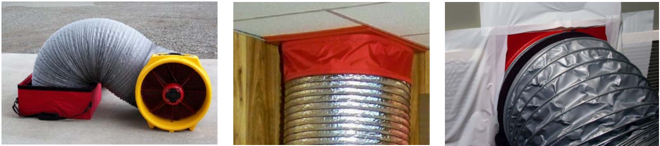
Figure 24. Flex duct for Door Fans (mainly used for enclosure integrity testing).
