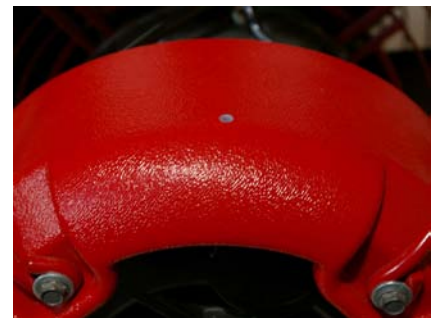
Figure 30. Pressure sensor on the fan motor casing.
