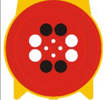
Range **C4**: ring A + B + center plate with 4 large + 4 small holes open.
