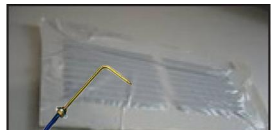
Figure 22: A Static Pressure Probe attached to a pressure tube allows the measurement of pressure without flow interference (e.g: inside a supply register)
