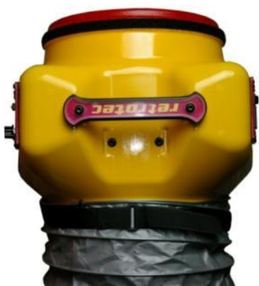
Figure 31: Install Flex Duct over the fan exhaust, for pressurization.
