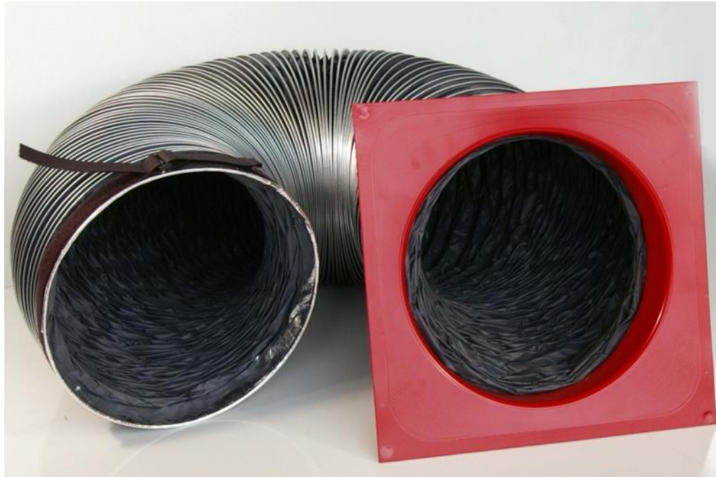
Figure 7: Flex Duct for duct testing system with Flange and strap.
