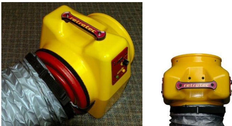
Figure 30: Install Flex Duct over the fan inlet, covering the Range Rings, for depressurization.
