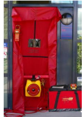
Figure 53: Blower Door system for testing tight enclosures.
