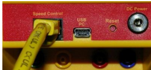
Figure 19: Electrical connections on the back of the gauge include Control Cable that goes to the DM-2 (shown connected), USB cable for a PC, reset switch and DC power connection.
