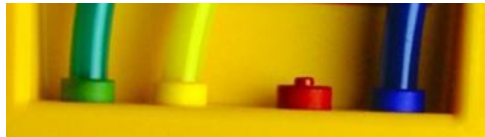
Figure 18: Pressure ports on the back of the gauge are color-coded to match the tubing.
