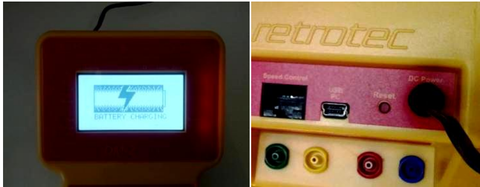
Figure 17: The screen and back view of the DM-2 while the batteries are being charged.
