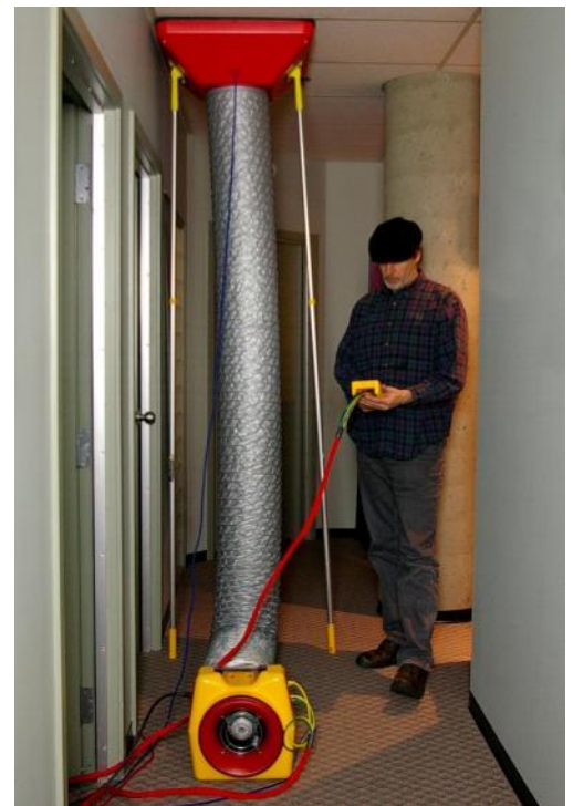
Figure 49: Measuring air flow with a Powered Flow Hood
