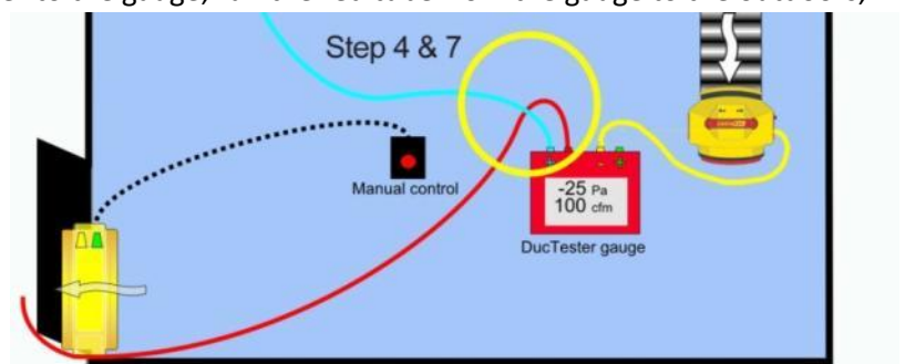
Figure 42: 1 Gauge Duct Leakage to Outdoors under depressurization, setting the duct pressure
