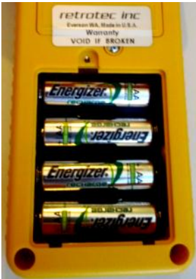
Figure 16: 4 NiMH AA batteries type in the battery compartment of the DM-2
