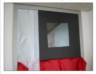
Alternatively, use a Calibration Plate in the optional second Fan Panel ,or, use the optional Flex Duct with a 400 sq. in. hole in a plate on the end.
