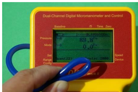
Figure 12. Errors in pressure reading from a pinched tube.
