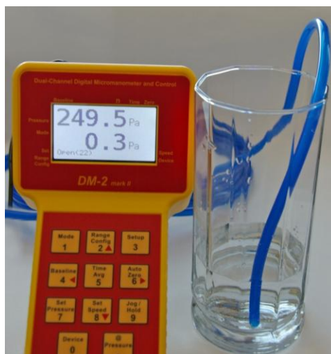
Figure 1. Gauge displaying 249.5 Pa (or 1 in WC).
