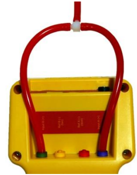
Figure 9. Fan Pressure check using a T-connection check.
