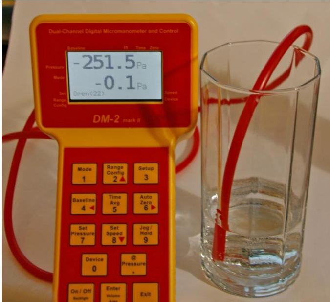
Figure 2. The gauge displays a negative pressure (-1 in WC, or -0.1 Pa) on the DM-2.
