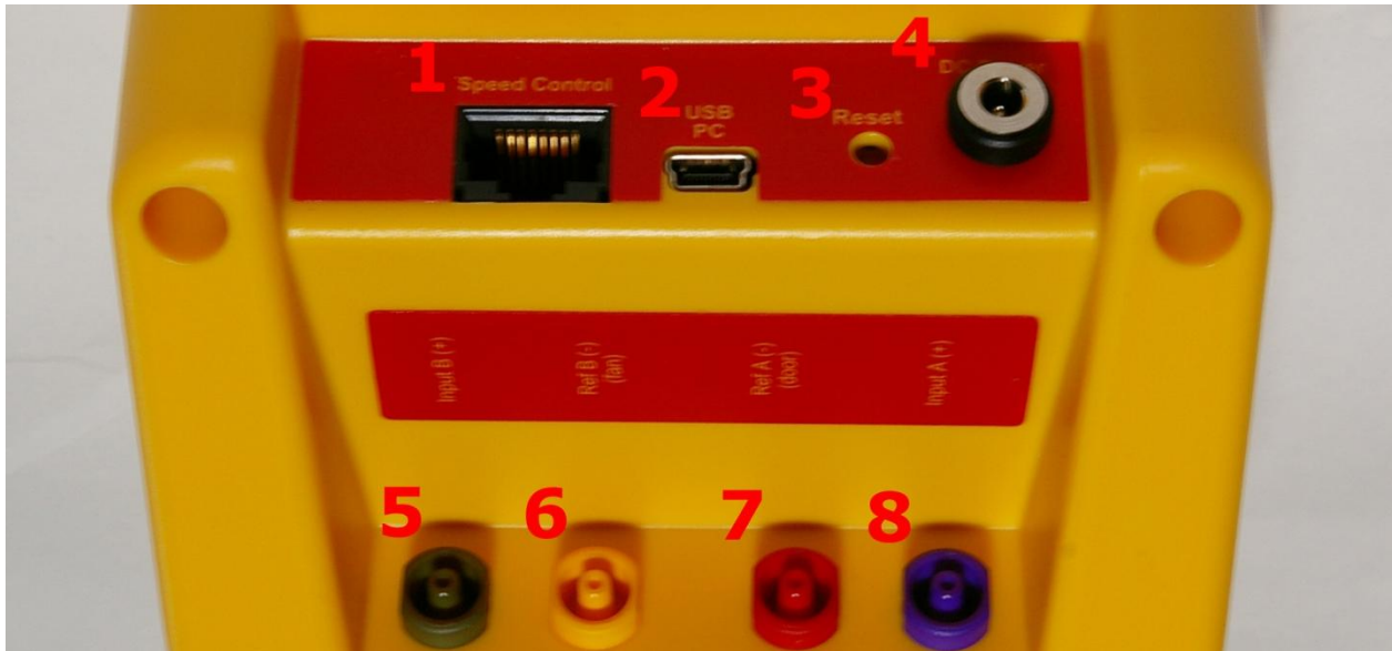
Figure 6. DM-2 back panel with pressure ports and electrical connections.
