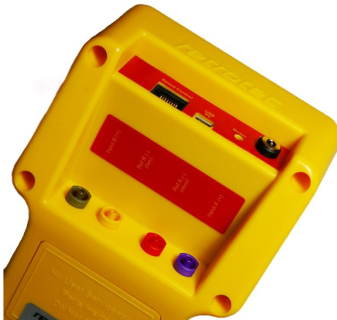
Figure 7. Pressure ports of the DM-2 gauge.
