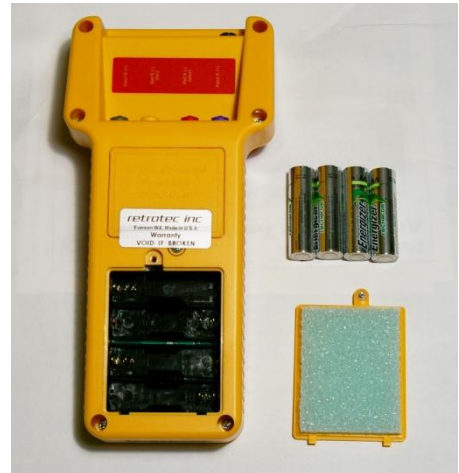
Figure 4 Battery cage and four rechargeable batteries for the DM-2.
